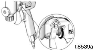
5. Using a small flat screwdriver, pry retaining ring off of trigger pin. Remove pin, washer, and trigger.
