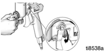
9. Remove plug and use small screwdriver to remove all components out front of gun.
