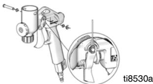
9. Pull trigger and replace nozzle.
