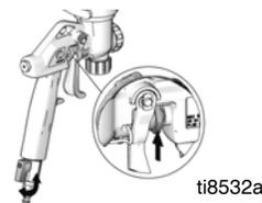
8. Insert pin through trigger and washers. Push the retaining clip onto the pin.
